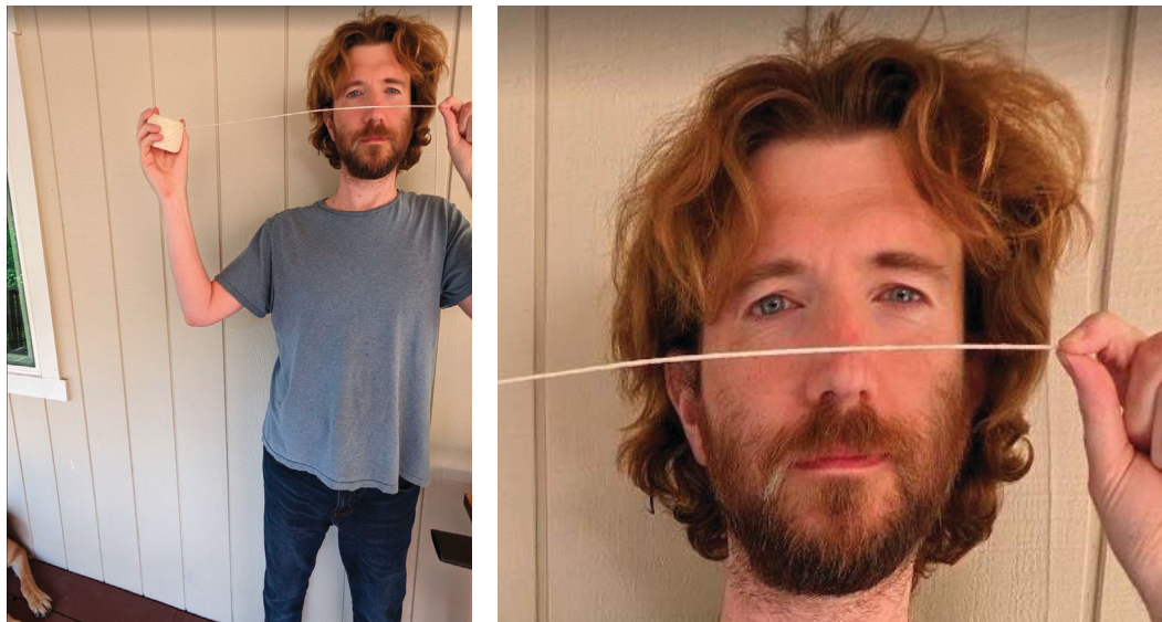
Figure 22. A taut piece of string in front of a face, photographed in the Google Pixel 5 camera app in ultrawide mode ( 0.5\times ). This app uses a version of Shih et al. (2019) , which is content-aware: the face is detected, and the region around it projected with stereographic projection, while the rest of the image uses linear perspective. As a result, the face does not exhibit marginal distortion as it would in linear perspective, but the piece of string is not straight, nor are the lines on the wall near the face. (Photo by Elena Adams.)
