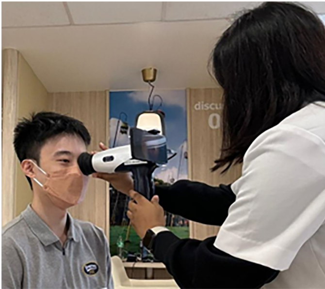
Figure 1. Demonstration of the image acquisition process using the smartphone-based oDocs Nun IR camera.
